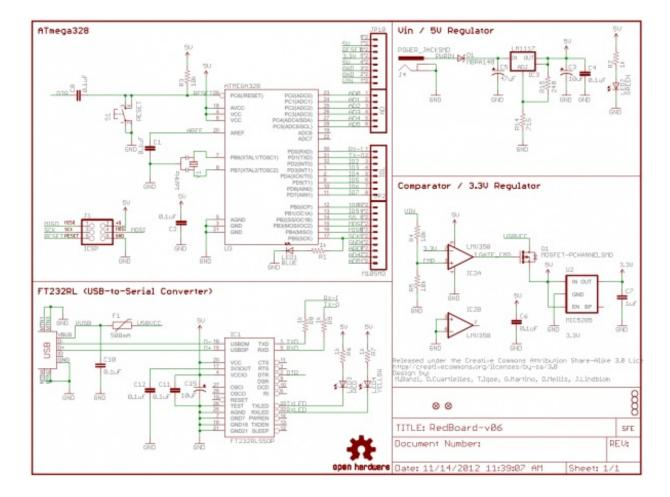
If the drawer of a schematic is really nice (like the engineer who designed this schematic for the RedBoard), they may separate sections of a schematic into logical, labeled blocks.
