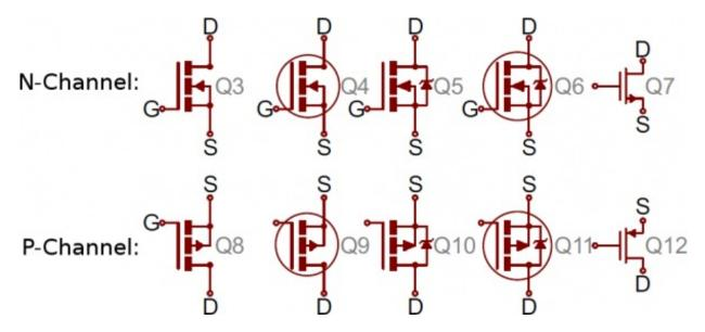
The arrow in the middle of the symbol (called the bulk) defines whether the MOSFET is n-channel or p-channel. If the arrow is pointing in means it's a n-channel MOSFET, and if it's pointing out it's a p-channel. Remember: "n is in" (kind of the opposite of the NPN mnemonic).
