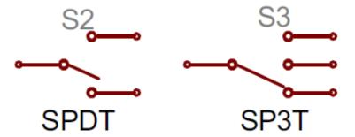
Switches with multiple poles, usually have multiple, alike switches with a dotted line intersecting the middle actuator.
