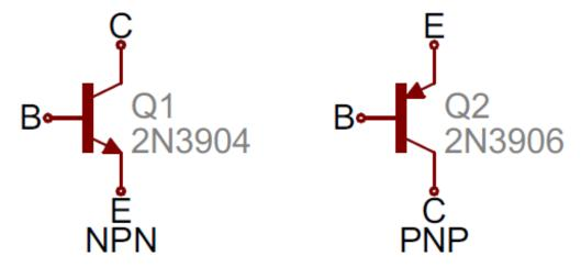
The collector (C) and emitter (E) pins are both in-line with each other, but the emitter should always have an arrow on it. If the arrow is pointing inward, it's a PNP, and, if the arrow is pointing outward, it's an NPN. A mnemonic for remembering which is which is "NPN: **not pointing in**."
