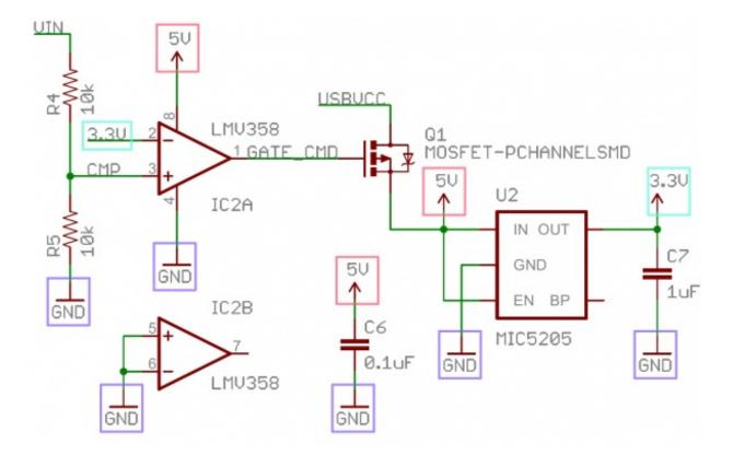
Like-named voltage nodes -- like GND, 5V, and 3.3V -- are all connected to their counterparts, even if there aren't wires between them.
