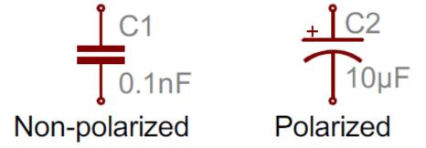
The symbol with one curved plate indicates that the capacitor is polarized. The curved plate usually Page 3 of 18
