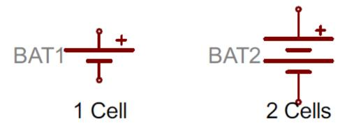
More pairs of lines usually indicates more series cells in the battery. Also, the longer line is usually used to represent the positive terminal, while the shorter line connects to the negative terminal.
