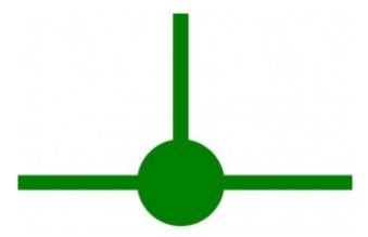
Nodes give us a way to say that "wires crossing this junction are connected". The absences of a node at a junction means two separate wires are just passing by, not forming any sort of connection. (When designing schematics, it's usually good practice to avoid these non-connected overlaps wherever possible, but sometimes it's unavoidable).
