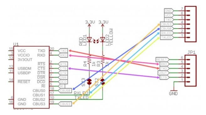
Each net with the same name is connected, as in this schematic for an FT231X Breakout Board. Names and labels help keep schematics from getting too chaotic (imagine if all those nets were actually connected with wires).
