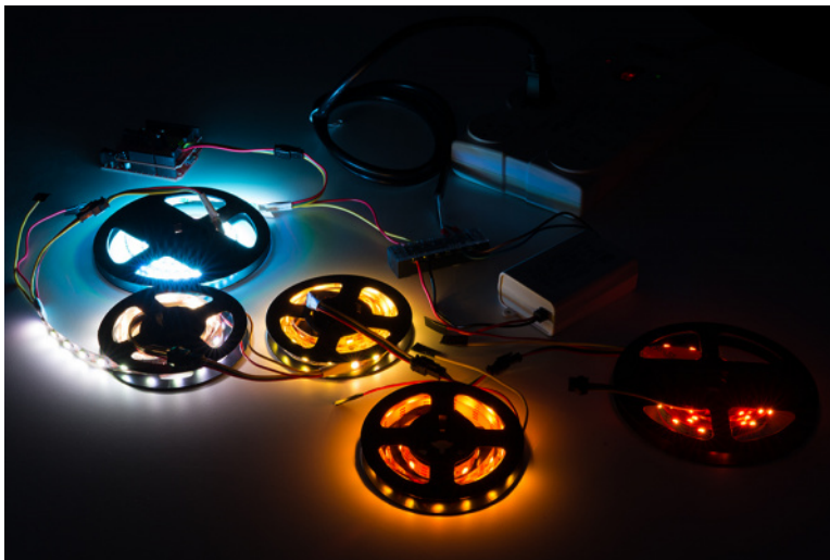
Voltage Drops Along the Daisy Chained LED Strips in Mean Well LED Switching Power Supply Hookup Guide: Power Large Loads and Daisy Chained LED Strips
