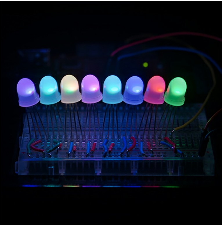
Diffused 8mm addressable LEDs connected on a breadboard.
