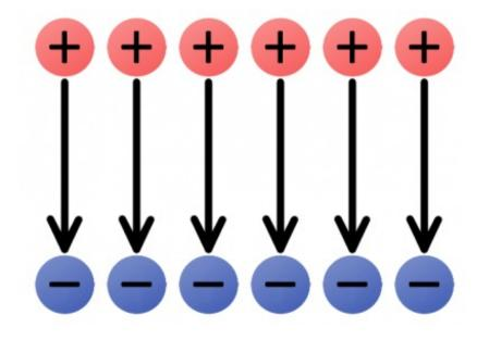
The uniform e-field above points away from the positive charges, towards the negatives. Imagine a tiny positive test charge dropped in the e-field; it should follow the direction of the arrows. As we've seen, electricity usually involves the flow of electrons--negative charges--which flow **against** electric fields.
