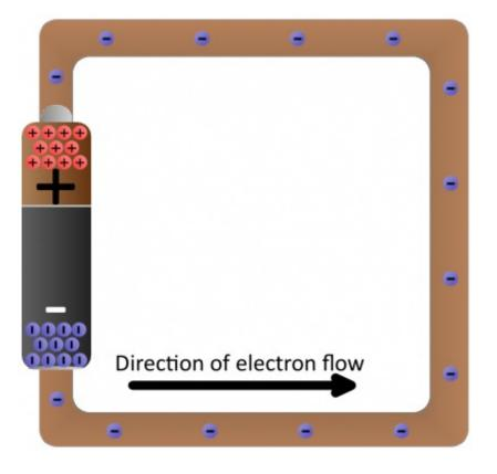
After a second of the current flow, the electrons have actually moved *very* little--fractions of a centimeter. However, the energy produced by the current flow is *huge*, especially since there's nothing in this circuit to slow down the flow or consume the energy. Connecting a pure conductor directly across an energy source is a **bad idea**. Energy moves very quickly through the system and is transformed into heat in the wire, which may quickly turn into melting wire or fire.
