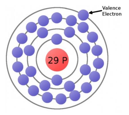
This is a copper atom diagram: 29 protons in the nucleus, surrounded by bands of circling electrons. Electrons closer to the nucleus are hard to remove while the valence (outer ring) electron requires relatively little energy to be ejected from the atom.
