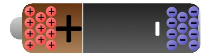
If we connected our wire full of conductive copper atoms to the battery, that electric field will influence the negatively-charged free electrons in the copper atoms. Simultaneously pushed by the negative terminal and pulled by the positive terminal, the electrons in the copper will move from atom to atom creating the flow of charge we know as electricity.
