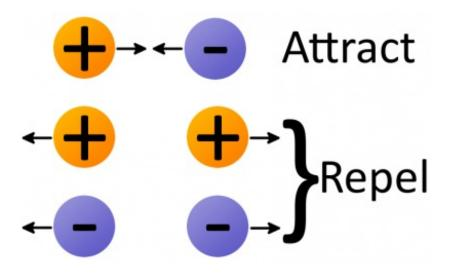
The **amount** of force acting on two charges depends on how far they are from each other. The closer two charges get, the greater the force (either pushing together, or pulling away) becomes.
