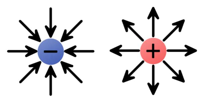
The electric fields of single charges. A negative charge has an inward electric field because it attracts positive charges. The positive charge has an outward electric field, pushing away like charges.
