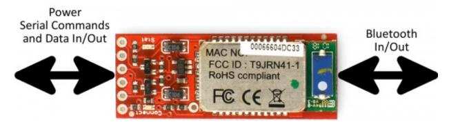
Establishing this data pipeline is a two step process. First, we need to connect something capable of sending and receiving serial data to the header of the Bluetooth modem. We achieved this in the <u>Hardware Hookup</u> phase by connecting an Arduino to the serial header, but any microcontroller with a UART could work. With the device connected we need to <u>configure the serial port</u> to work at the same baud rate the the modem is configured to -- they default to **115200 bps** (8-N-1).
