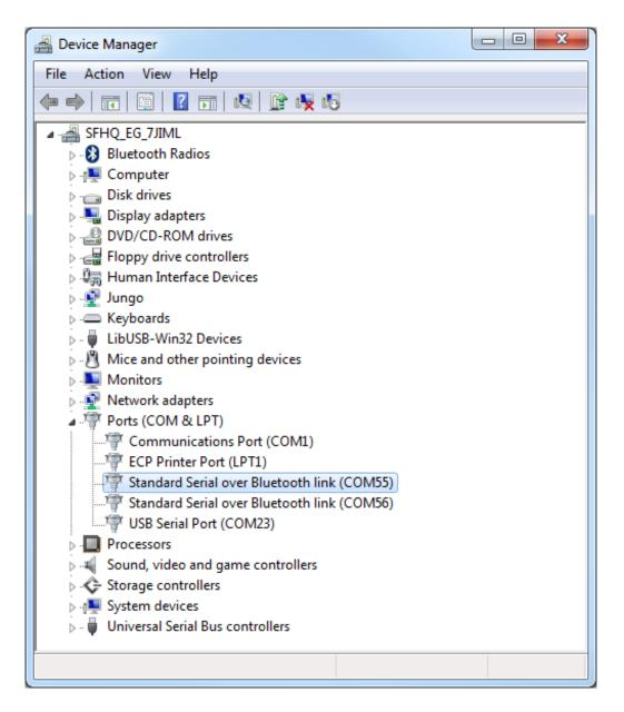
To open up a connection between the Bluetooth devices, open up a terminal to that COM port at 9600 bps (8-N-1). (If you see two ports, try the lower number first). When the terminal opens up, your Bluetooth modem's green connect LED should light up. Connection successful!
