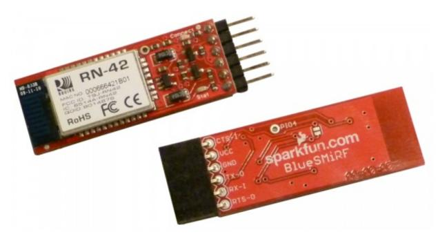
Right-angle male or female headers are good options for assembly. They make the modules breadboard or jumper-wire compatible.
