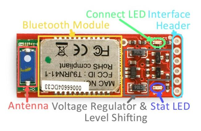
Finally, be aware of where the antenna is -- give it some room to breathe. Don't place it near any big chunks of metal or enclose it in a Faraday cage, and you should be just fine.
