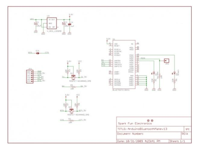
Key to the design are **level shifting circuits** between the RN-41/42's serial pins, and the output header. The maximum operating voltage of the Roving Networks modules is 3.3V, so these enable a device operating at 5V (like an Arduino) to safely communicate with the Bluetooth modems. There is also a linear 3.3V regulator on the board, so a voltage from 3.3V to 6V can be used to supply power to the module.
