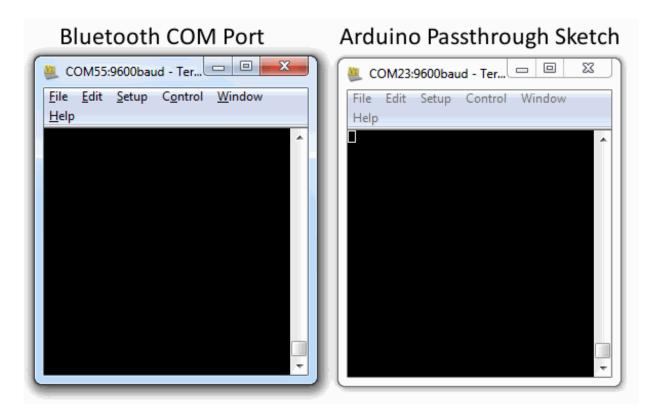
If you're within the config timer window (cycle power on the modem if you're not), you can even *remotely* enter command mode by sending the "\$\$\$" string. Now you can remotely alter the settings of your Bluetooth modem. Nifty!
