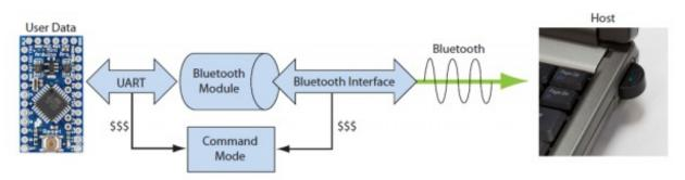
**To enter command mode** from data mode, the host controller needs to send a string of three\$ symbols (\$\$\$).
