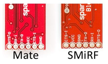
The pinout of the Mate matches that of products like the <u>FTDI Basic</u> and the <u>FTDI Cable</u>. It's a "standardized" pinout for a serial interface and power supply combination. This pinout allows the Mate to be plugged directly into the serial header of <u>Arduino Pro's</u> and <u>Pro Minis</u>.
