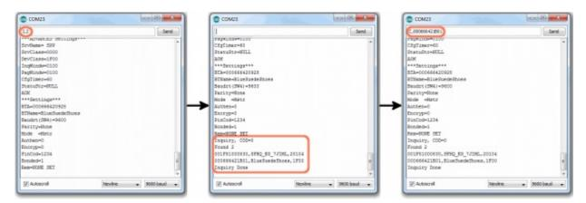
If the modem finds any modules, you can try sending the **connect command** -- C,<address> -- to Page 17 of 25 connect to one of them. The modem in the example above found two devices in range, by sending the C,000666421B01 command, we can attempt to connect to one of them.
