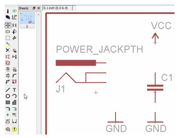
The hard part, sometimes, is identifying which part on a circuit symbol is actually a pin. Usually they're recognizable by a thin, horizontal, red line off to the side of a part. Sometimes (not always) they're labeled with a pin number. Make sure you click on the very end of the pin when you start or finish a net route.
