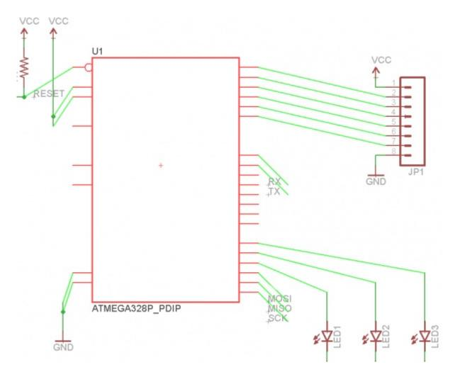
If all the nets connected to a part MOVE with it, all connections are good.
