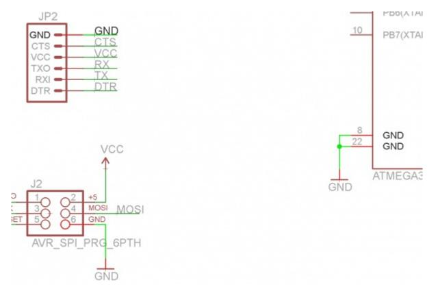
As an alternative to show, you can temporarily MOVE a part a part to make sure nets are connected to it. Use MOVE to pick a part up, and the nets connected to it should bend and adjust to remain so. Just make sure you hit ESC to *not* move the part (or UNDO if you accidentally move it).
