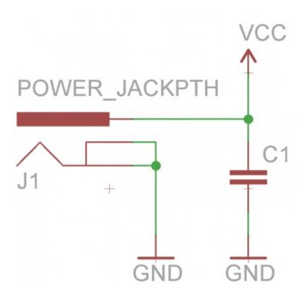
Whenever a net splits in two directions a**junction node** is created. This signifies that all three intersecting nets *are* connected. If two nets cross, but there's not a junction, those nets*are not* connected.
