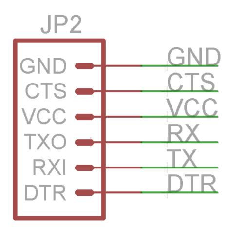
VCC should be the only other net that warns you that you'll be connecting to other nets named "VCC" (anything connected to a VCC voltage node). For the other named nets, we'll need to create this same stub somewhere else. Where exactly? Well, we need to add a "RX" and "TX" net on the ATmega328, and a "DTR" nearby as well:
