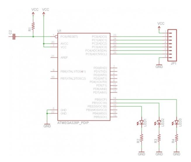
Don't forget to add nets between the LEDs, resistors, and GND symbols!
