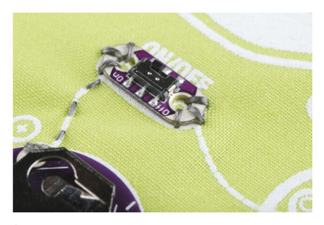
Conductive thread can carry current the same way that wires can, which means it can be used to create a circuit. This allows the user to sew a circuit together, creating flexible circuits that require no soldering. In some textile-based projects, this is the most practical tool to maintain the hang of the fabric. Educationally, it's a very safe and unintimidating way to learn how to use embedded electronics.
