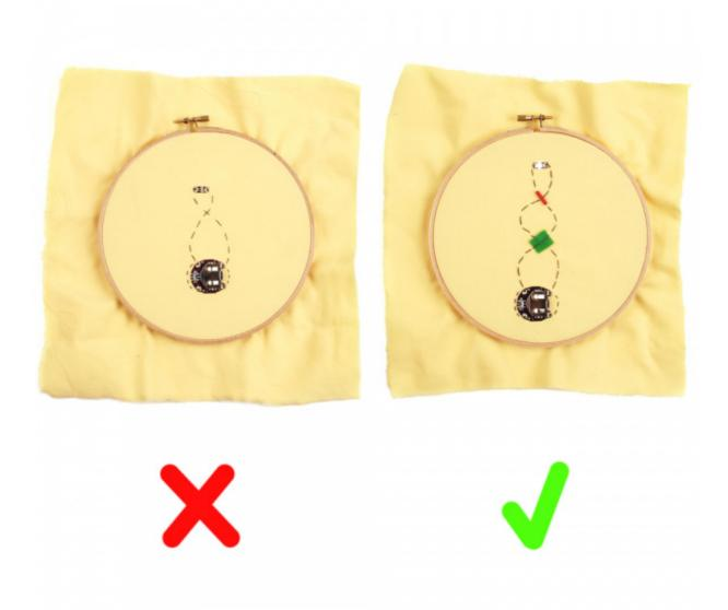
To add a little additional protection from accidental shorts, you can wax the entire length of your thread before you begin sewing. This will help smooth down stray fibers as well as coating the thread with a thin layer of insulating wax. It's not enough to truly insulate, but it will make it far less likely that two threads come into contact and immediately cause a short.
