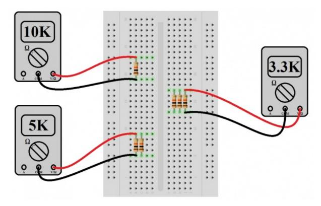
Repeat the exercise now with 3, 4 and 5 resistors. The calculated/measured values should be  $3.33k\Omega$ ,  $2.5k\Omega$  and  $2k\Omega$ , respectively. Did everything come out as planned? If not, go back and check your connections. If it did, EXCELSIOR! Go have a milkshake before we continue. You've earned it.
