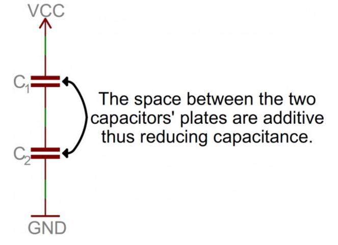
Remember that in a series circuit there's only one path for current to flow. It follows that the number of electrons that are discharging from the cap on the bottom is going to be the same number of electrons coming out of the cap on the top. So the capacitance hasn't increased, has it?
