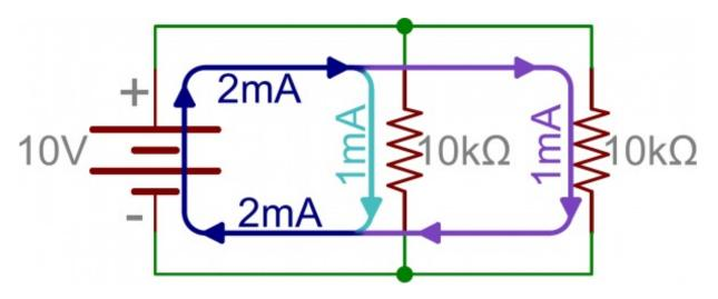
While we can say that  $10k\Omega \parallel 10k\Omega = 5k\Omega$  ("||" roughly translates to "in parallel with"), we're not always going to have 2 identical resistors. What then?
