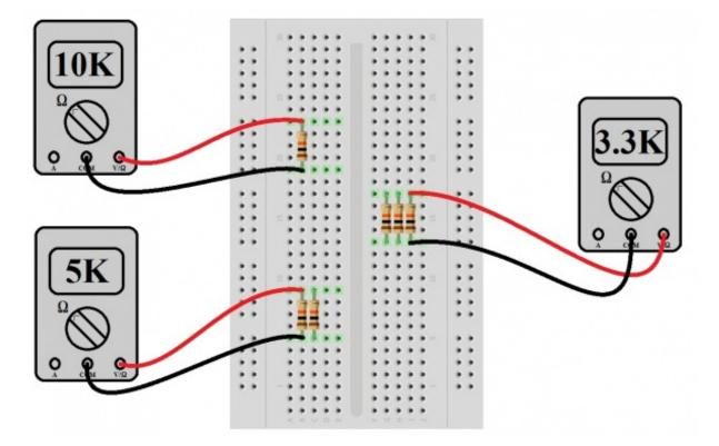
Repeat the exercise now with 3, 4 and 5 resistors. The calculated/measured values should be  $3.33k\Omega$ ,  $2.5k\Omega$  and  $2k\Omega$ , respectively. Did everything come out as planned? If not, go back and check your connections. If it did, EXCELSIOR! Go have a milkshake before we continue. You've earned it.
