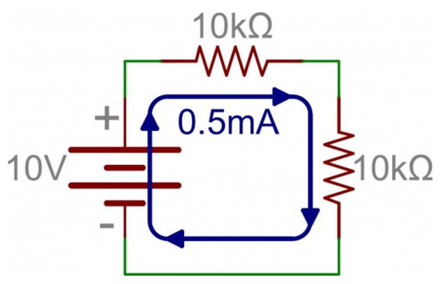
In other words, there's still only one path for current to take and we just made it even harder for current to flow. How much harder?  $10k\Omega + 10k\Omega = 20k\Omega$ . And, that's how we calculate resistors in series -- just **add their values**.
