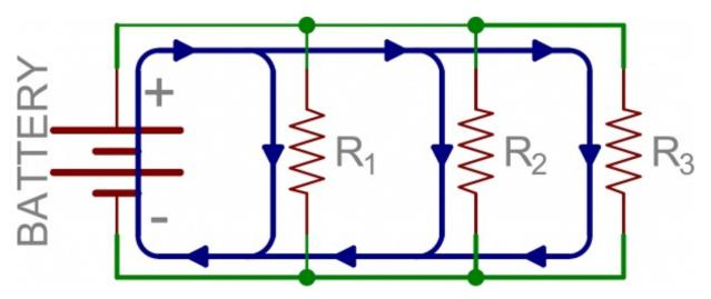
From the positive battery terminal, current flows to  $R_1$ ... and  $R_2$ , and  $R_3$ . The node that connects the battery to  $R_1$  is also connected to the other resistors. The other ends of these resistors are similarly tied together, and then tied back to the negative terminal of the battery. There are three distinct paths that current can take before returning to the battery, and the associated resistors are said to be in parallel.
