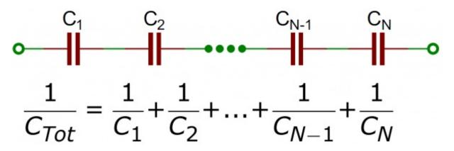
It may seem that there's no point to adding capacitors in series. But it should be pointed out that one thing we did get is twice as much voltage (or voltage ratings). Just like batteries, when we put capacitors together in series the voltages add up.
