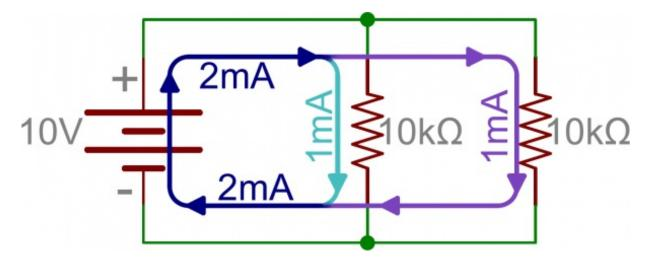
While we can say that  $10k\Omega \parallel 10k\Omega = 5k\Omega$  ("||" roughly translates to "in parallel with"), we're not always going to have 2 identical resistors. What then?
