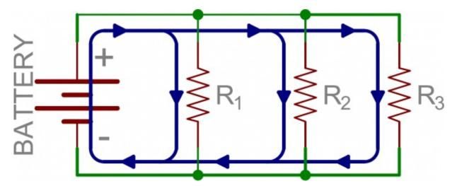
From the positive battery terminal, current flows to  $R_1$ ... and  $R_2$ , and  $R_3$ . The node that connects the battery to  $R_1$  is also connected to the other resistors. The other ends of these resistors are similarly tied together, and then tied back to the negative terminal of the battery. There are three distinct paths that current can take before returning to the battery, and the associated resistors are said to be in parallel.
