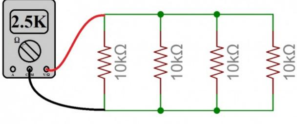
Total Resistance = Value of One Resistor / Number of Resistors 2.5K = 10K / 4
