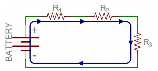
There's only one way for the current to flow in the above circuit. Starting from the positive terminal of the battery, current flow will first encounter  $R_1$ . From there the current will flow straight to  $R_2$ , then to  $R_3$ , and finally back to the negative terminal of the battery. Note that there is only one path for current to follow. These components are in series.
