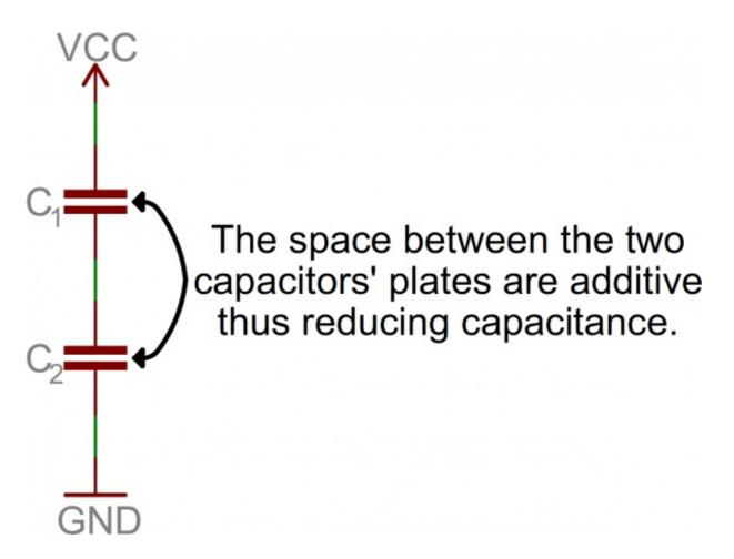
Remember that in a series circuit there's only one path for current to flow. It follows that the number of electrons that are discharging from the cap on the bottom is going to be the same number of electrons coming out of the cap on the top. So the capacitance hasn't increased, has it?
