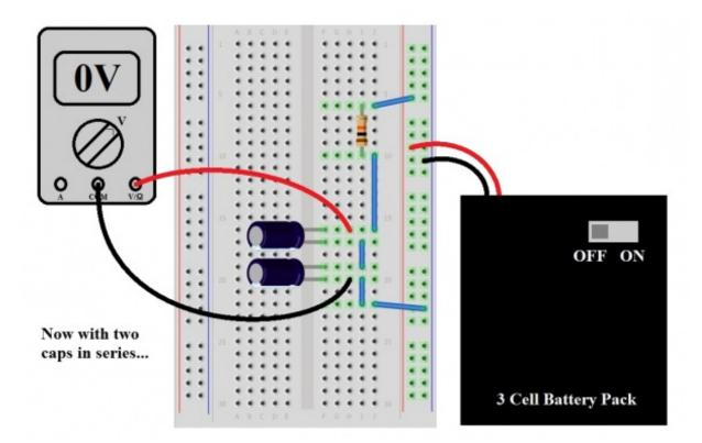
With that in mind, plug in another capacitor in series with the first, make sure the meter is reading zero volts (or there-abouts) and flip the switch to "ON". Did it take about half as much time to charge up to the battery pack voltage? That's because there's half as much capacitance. The electron gas tank got smaller, so it takes less time to charge it up. A third capacitor is suggested for this experiment just to prove the point, but we're betting the reader can see the writing on the wall.
