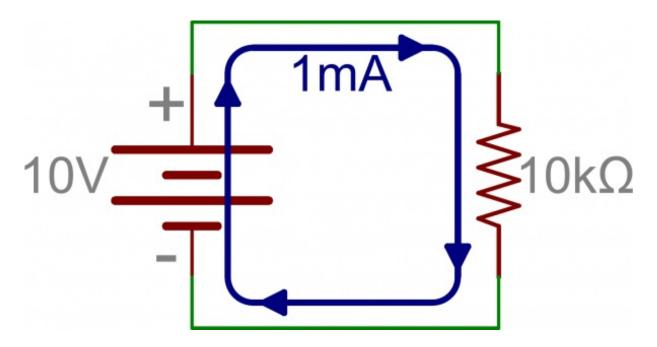
If we then put another  $10k\Omega$  resistor in series with the first and leave the supply unchanged, we've cut the current in half because the resistance is doubled.
