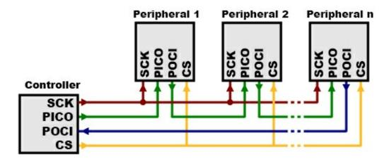
Note that, for this layout, data overflows from one peripheral to the next, so to send data to anyone peripheral, you'll need to transmit enough data to reach *all* of them. Also, keep in mind that the *first* piece of data you transmit will end up in the *last* peripheral.
