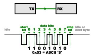
(By the way, if you noticed that "11001010" does not equal 0x53 in the above diagram, kudos to your attention to detail. Serial protocols will often send the least significant bits first, so the smallest bit is on the far left. The lower nybble is actually 0011 = 0x3, and the upper nybble is 0101 = 0x5.)
