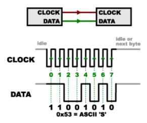
One reason that SPI is so popular is that the receiving hardware can be a simple<u>shift register</u>. This is a much simpler (and cheaper!) piece of hardware than the full-up UART (Universal Asynchronous Receiver / Transmitter) that asynchronous serial requires.
