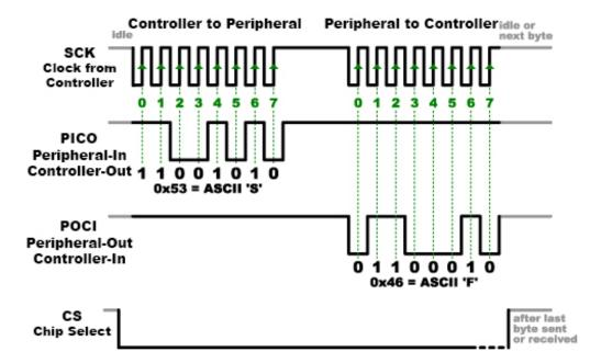
The CS line is normally held high, which disconnects the peripheral from the SPI bus. (This type of logic is known as "active low," and you'll often see used it for enable and reset lines.) Just before data is sent to the peripheral, the line is brought low, which activates the peripheral. When you're done using the peripheral, the line is made high again. In a <u>shift register</u>, this corresponds to the "latch" input, which transfers the received data to the output lines.
