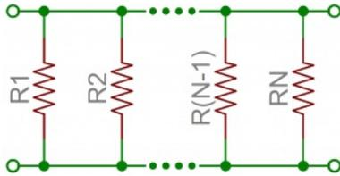
$$\frac{1}{R_{tot}} = \frac{1}{R_1} + \frac{1}{R_2} + \dots + \frac{1}{R_{N-1}} + \frac{1}{R_N}$$
