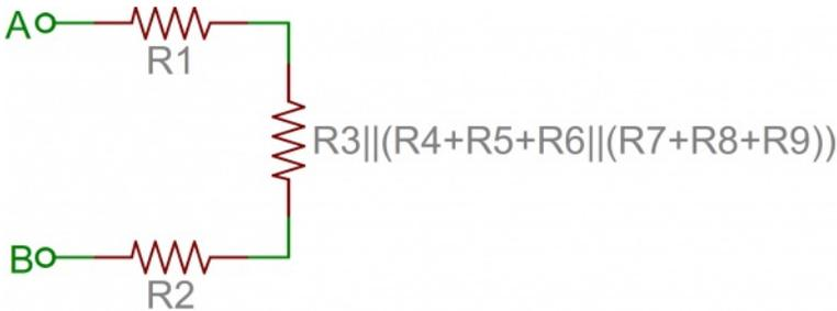
And that's just three series resistors between the  $A$  and  $B$  terminals. Add 'em up! So the total resistance of that circuit is:  $R_1 + R_2 + R_3 \parallel (R_4 + R_5 + R_6 \parallel (R_7 + R_8 + R_9))$ .
