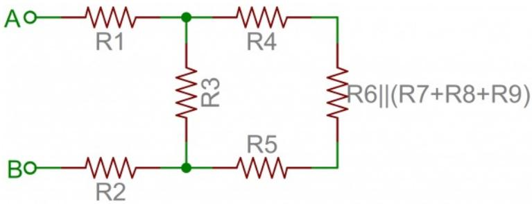
Now the four right-most resistors can be simplified even further.  $R_4$ ,  $R_5$  and our conglomeration of  $R_6 - R_9$  are all in series and can be added. Then those series resistors are all in parallel with  $R_3$ .
