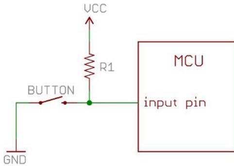
In the circuit above, when the switch is open the MCU's input pin is connected through the resistor to 5V. When the switch closes, the input pin is connected directly to GND.
