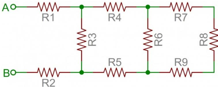
To solve such a problem, start at the back-end of the circuit and simplify towards the two terminals. In this case  $R_7$ ,  $R_8$  and  $R_9$  are all in series and can be added together. Those three resistors are in parallel with  $R_6$ , so those four resistors could be turned into one with a resistance of  $R_6 || (R_7 + R_8 + R_9)$ . Making our circuit:
