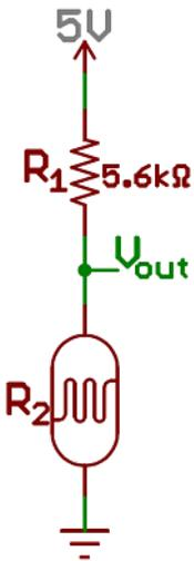
Here a resistor  $R_1$  and a photocell create a voltage divider to create a variable voltage output.
