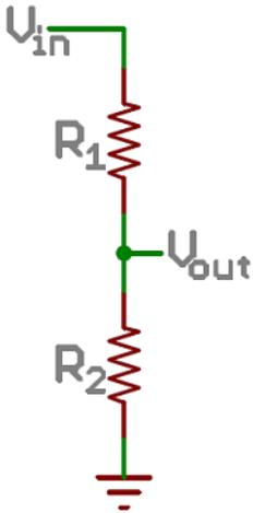
Two resistors,  $R_1$  and  $R_2$ , are connected in series and a voltage source ( $V_{in}$ ) is connected across them. The voltage from  $V_{out}$  to GND can be calculated as:
