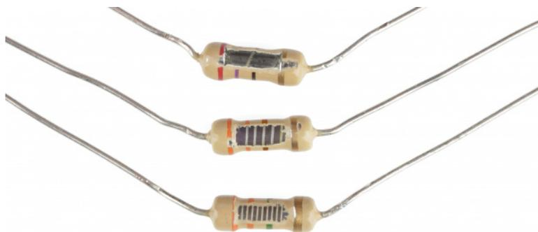
Peek inside the guts of a few carbon-film resistors. Resistance values from top to bottom:  $27\Omega$ ,  $330\Omega$  and a  $3.3M\Omega$ . Inside the resistor, a carbon film is wrapped around an insulator. More wraps means a higher resistance. Pretty neat!
