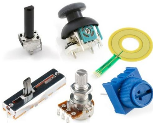
A smattering of potentiometers. From top-left, clockwise: [a standard 10k trimpot](#), [2-axis joystick](#), [softpot](#), [a breadboard friendly 10k trimpot](#), [classic right-angle](#), and [a slide pot](#).
