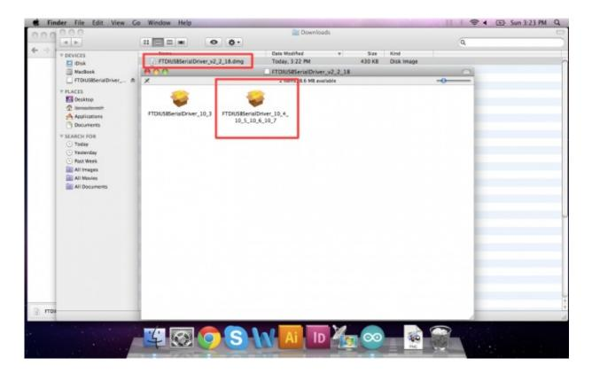
In short, the process involves heading over to the FTDI driver website, and downloading the most up-to-date VCP drivers. Then you'll simply run the "FTDIUSBSerialDriver\_v2\_2\_18.dmg" file you downloaded, and follow the installation prompts.
