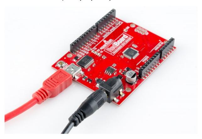
It is acceptable to connect both a barrel jack and a USB connector at the same time. The RedBoard has power-control circuitry to automatically select the best power source.
