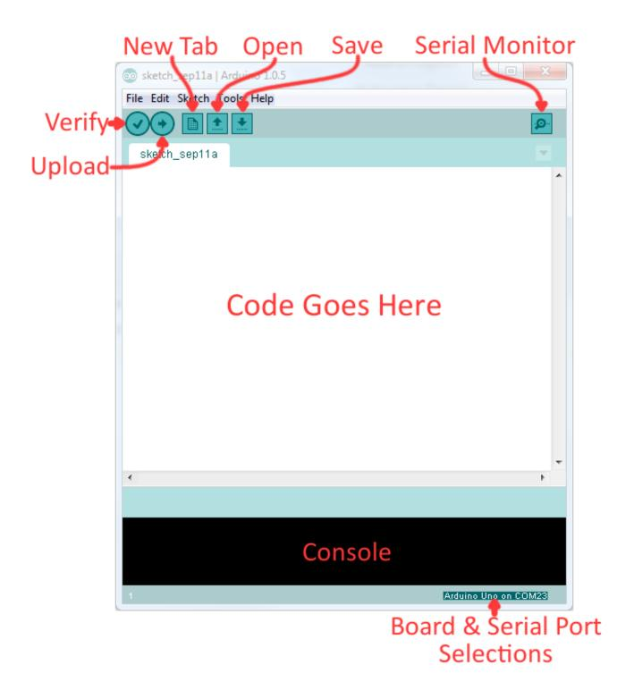
Lets upload a **Blink sketch** to make sure our new RedBoard setup is totally functional. Go up to the **File** menu in Arduino, then go to **Examples > 01.Basics > Blink** to open it up.
