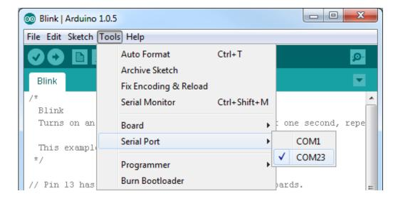
If you've got more than one port, and you're not sure which of the serial ports is your RedBoard, unplug it for a moment and check the menu to see which one disappears.
