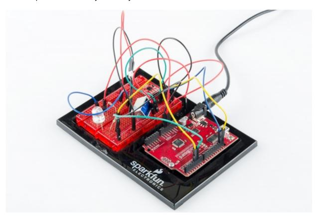
A tangled assortment of <u>jumper wires</u> run between the RedBoard headers and components on a <u>breadboard</u>. An <u>Arduino baseplate</u> holds them all in one place.
