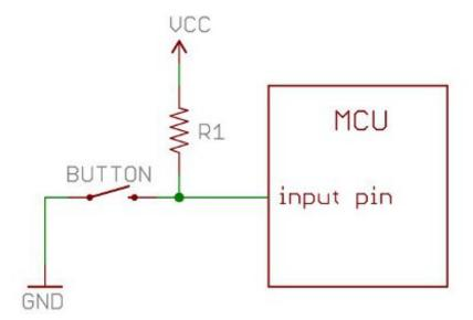
Let's say you want to limit the current to approximately 1mA when the button is pressed in the circuit above, where Vcc = 5V. What resistor value should you use?
