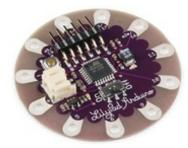
The <u>LilyPad Arduino Simple</u> is the brains of the ProtoSnap's operation. The heart of this board is that tiny black <u>chip</u> in the center – an**ATmega328 microprocessor**. A microprocessor is a tiny computer that can be programmed to interact with the LEDs, buzzers, and many other peripherals. The ATmega328 is one of our favorite microcontrollers - it's got a good set of inputs and outputs, lots of features, and it plays very nicely with the Arduino software.
