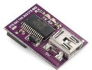
This board serves three separate purposes. First of all, it canpower the LilyPad Arduino Simple. A <u>power source</u> for your project is one of the most important decisions you'll make. The FTDI Basic will source power from your computer's USB port, and relay it over to the LilyPad Arduino.
