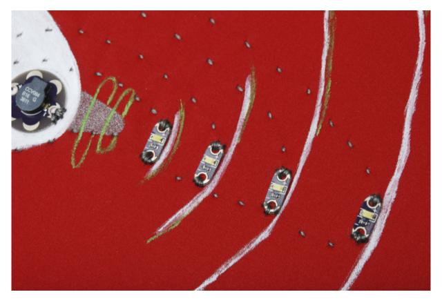
Continue this trace down and around to the negative pin of the Arduino. I neglected to get a picture
