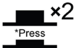
Pro Micro and Fio v3 Pro Micro, Fio v3, and any SparkFun Atmega32U4-based board reset functionality. Press reset twice, quickly to enter bootloader mode.
