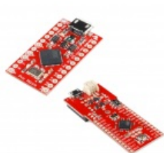
Pro Micro and Fio v3 Pro Micro, Fio v3, and any SparkFun Atmega32U4-based board reset functionality. Press reset twice, quickly to enter bootloader mode.
