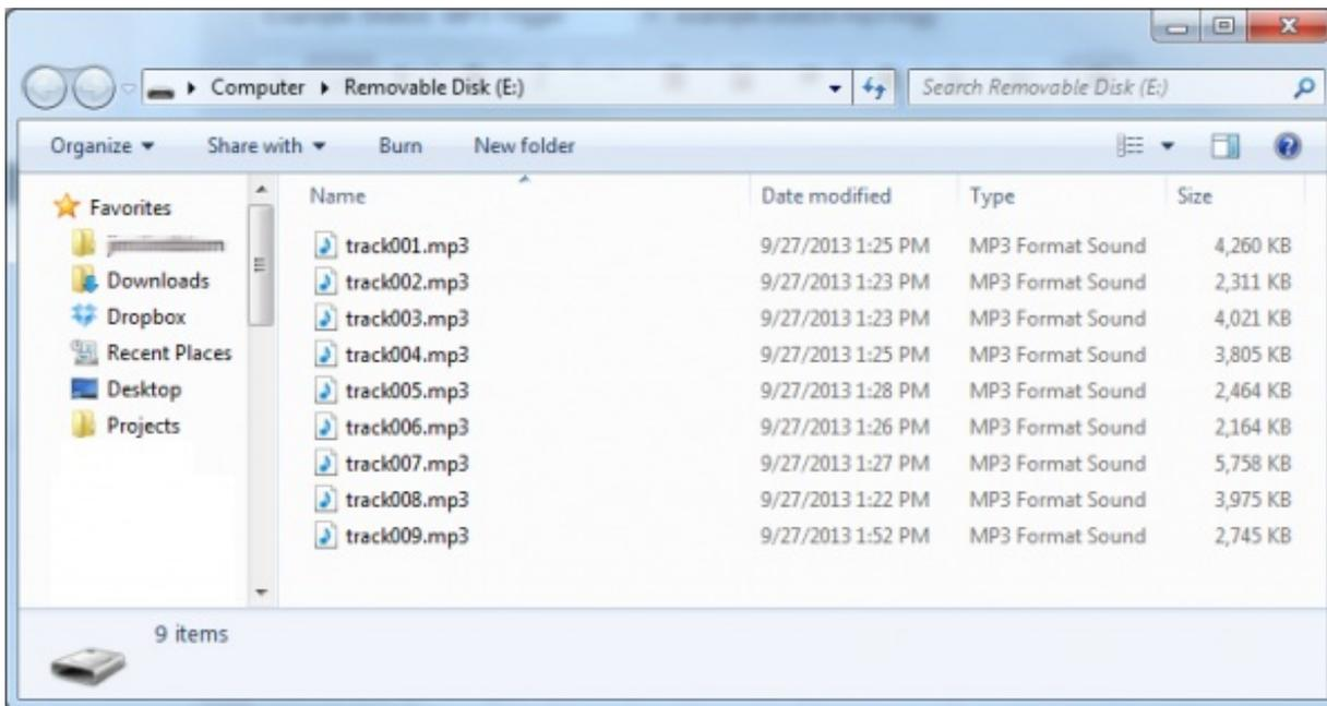
The first trigger -- D0 -- will play an MP3 named "track001.mp3", the second trigger -- D1 -- will play "track002.mp3", and so on up to A4 which will play "track009.mp3".
