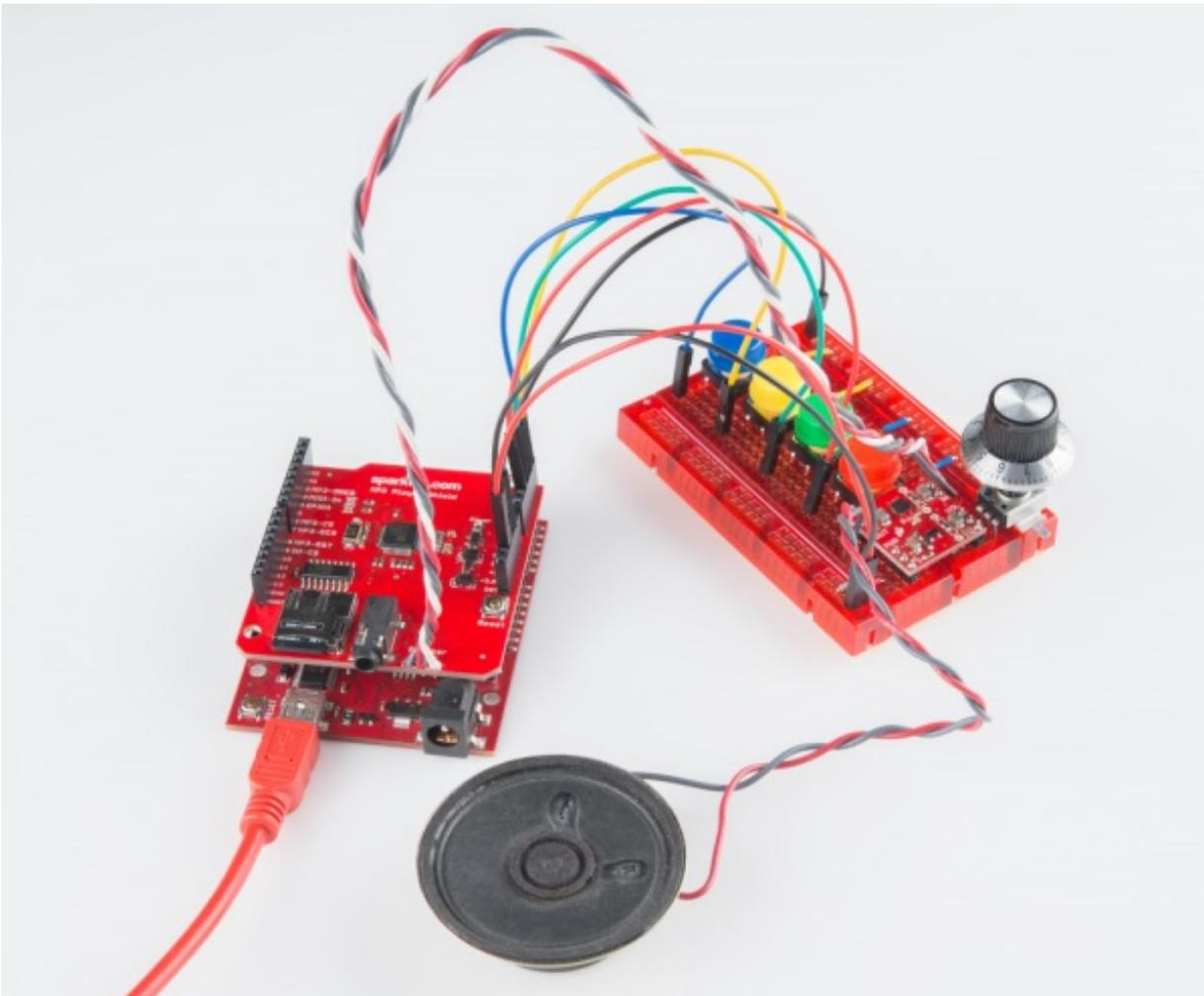
You can either plug headphones into the on-board jack to listen, or, if you want to get fancy with it, use the three broken out "Speaker" pins. Here's our setup with a combination of [MonoAmp Breakout](#) and [8  \$\Omega\$  Speaker](#):
