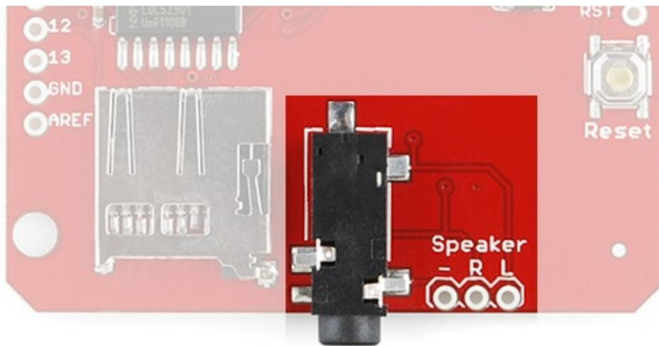
The right and left channels, as well as the audio ground are also broken out to a **0.1" header** next to the headphone jack. You can use these pins to connect up to a speaker or amplifier input.
