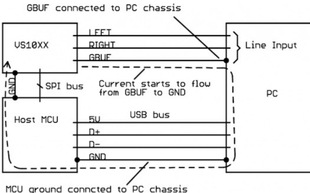
Figure 6: Ground loop is formed when GBUF and USB is connected to PC ground
