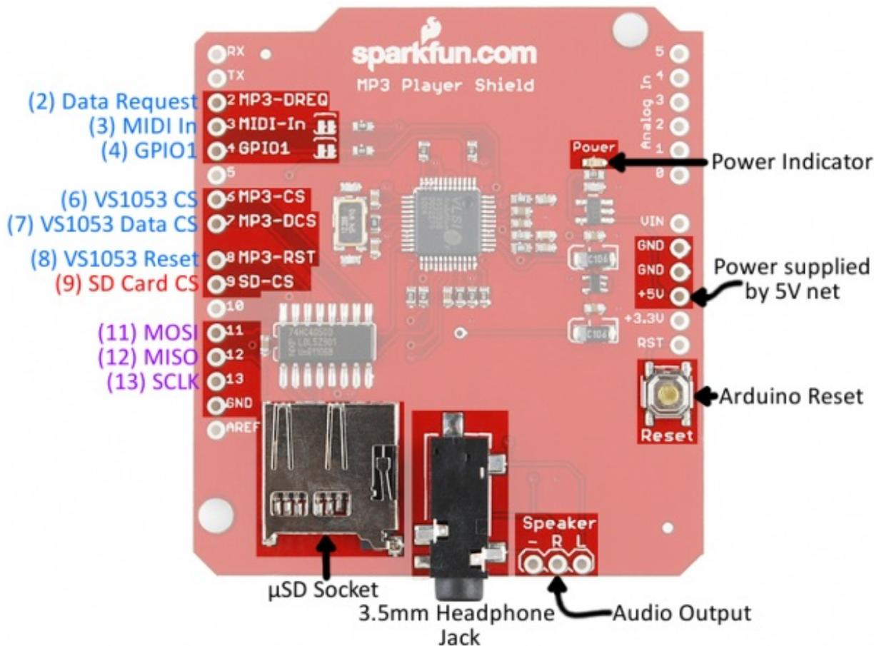
In the image above, the blue labels are pins used by the VS1053 MP3 Codec IC, the red labels are used for communication with the μSD card, and the purple-labeled pins are used by *both* components (yay [SPI!](#)).
