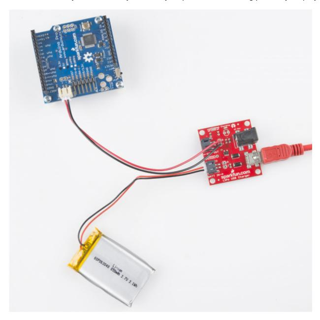
You can use the "SYS OUT" header to power a<u>3.3V Arduino Pro</u>. All while leaving your battery connected to the charger.
