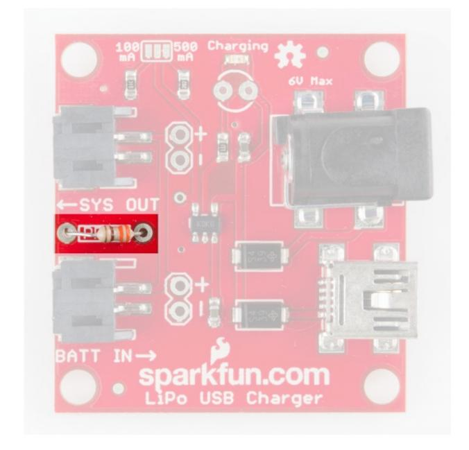
Before adding the resistor, **disconnect both jumpers** discussed in the section above. Then use this equation to select your resistor:
