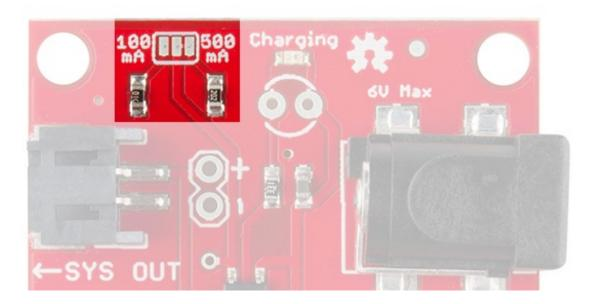
If you look *really* closely at that jumper, you may see a small trace connecting the middle pad to the 500mA-labeled outer pad. As such, this board is **configured to deliver a 500mA current by default**.
