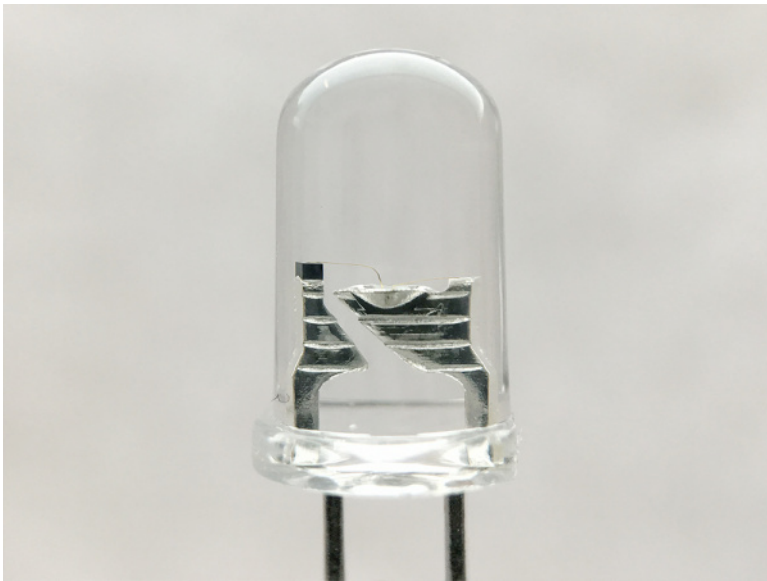
LED with Built-In Resistor Close Up
