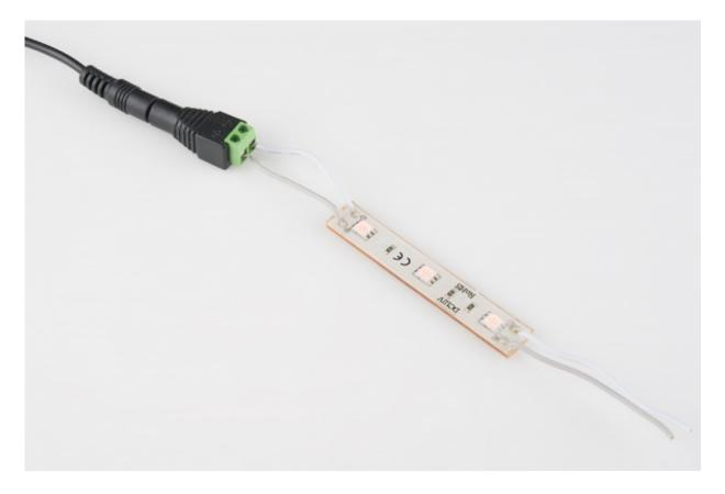
The <u>DC Barrel Jack Screw Terminal Adapter</u> makes connecting the 12V wall wart to the LED bar way easy.
