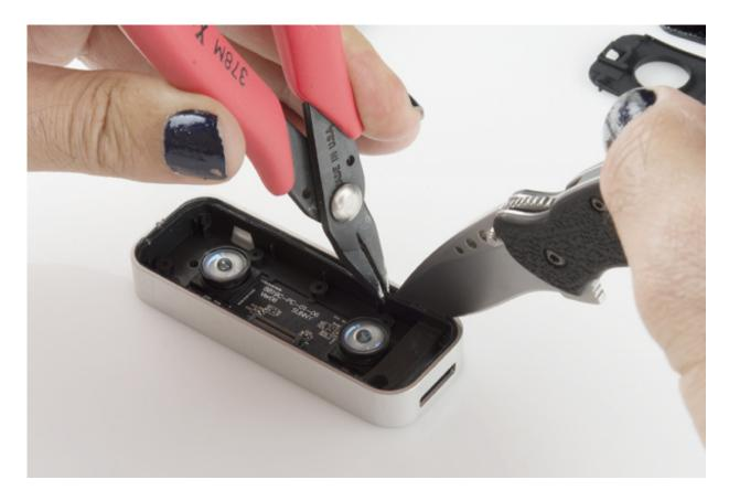
I gave extracting the cradle a try, but it didn't come easily--probably glued in. If you'll remember back to first post-peeling screws I discovered--the ones coming up from the bottom--you can now see what they were holding down. Odd that they felt like screws *and* glue were needed, but that's in keeping with the quality assembly elsewhere in the design.
