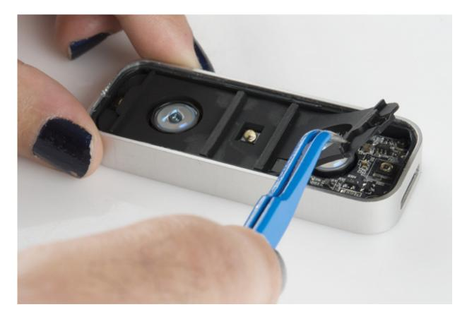
Peeling away the rubber baffle (which is glued, lightly, to the PCB underneath) reveals the top of a two-sided PCB. The top side is mostly bookkeeping: power supplies, the LED drivers, the LEDs themselves. There are three points of interest, however.
