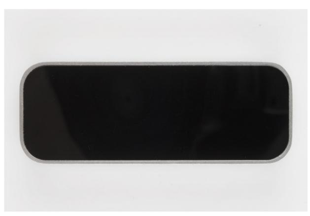
The top surface has the sort of coloration that suggests infrared transparency. It's mildly flexible to the touch, so we know it's plastic. It's also absolutely perfect for attracting and holding smudges, but the software will actually **warn** you that there's a smudge on the surface, and that's pretty dang cool.
