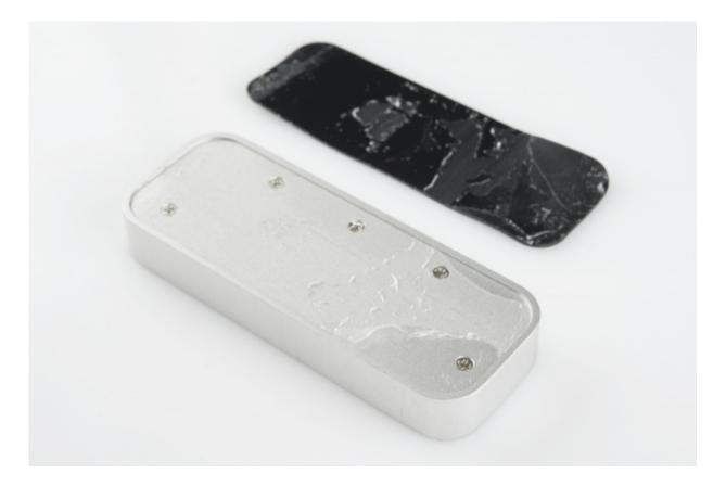
Beneath, I found five tiny screws. Bonus points to the Leap Motion folks for not using tamperresistant screws- I really appreciate that! A Philips 0 screwdriver took the screws right out, and that didn't do squat as far as improving access to more innards was concerned. We'll see why that is in a bit.
