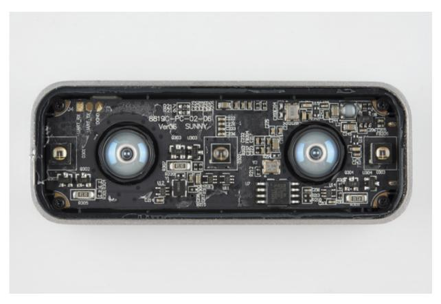
In the upper left corner, you can see a three-point serial port- RX, TX and GND. I didn't dig into it too
