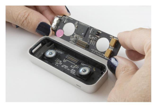
After I removed those screws, the top board lifted out easily, revealing another board and a surprising amount of empty space.
