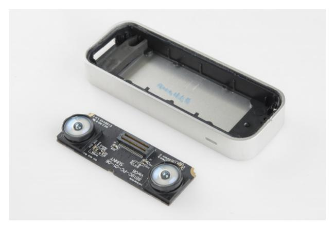
Once I managed to get the PCB out, you can see that there's not much else going on in there. The cradle and the soft-rubber spacer seem to be pretty standard--they don't appear to be conductive material or anything fancy like that. The board itself has the bare-copper corners we saw on the top board, even though there were no screws holding those corners down.
