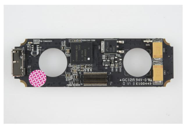
The back side of the top PCB has fewer, but larger, components: two large tantalum capacitors to guard against power supply brown-out during surge currents, a large surface-mount MOSFET
