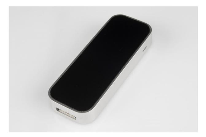
Seamless, glossy, and totally devoid of visible fasteners, the Leap Motion has the brushedaluminum minimalist design which is the new "bent-sheet-metal-and-beige-plastic" aesthetic. The only notable external features are a tiny diffused plastic LED indicator window and data port on one end.
