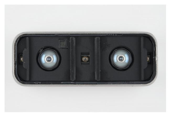
In the top-down view, you can see some interesting things. First off, the rubber sheet is clearly design to baffle the light, stopping light bouncing around inside the chassis from reaching the
