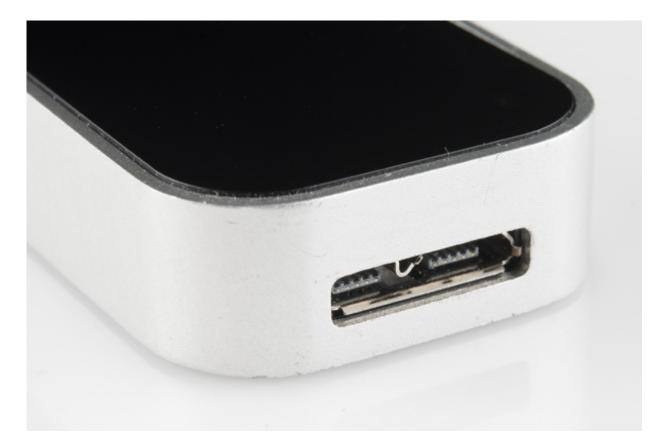
The Leap is tiny- 6.2mm thick, 25mm wide and 75mm long. At one end you'll find the data port- a <u>USB 3.0</u> micro-B connector. While it **can** be used as a 3.0 device, I found it worked just fine with a standard USB micro-B connector, plugged into a USB 2.0 port. I'm guessing that chokes your framerate a bit, but I was still seeing framerates up near 200fps, which is pretty darn good.
