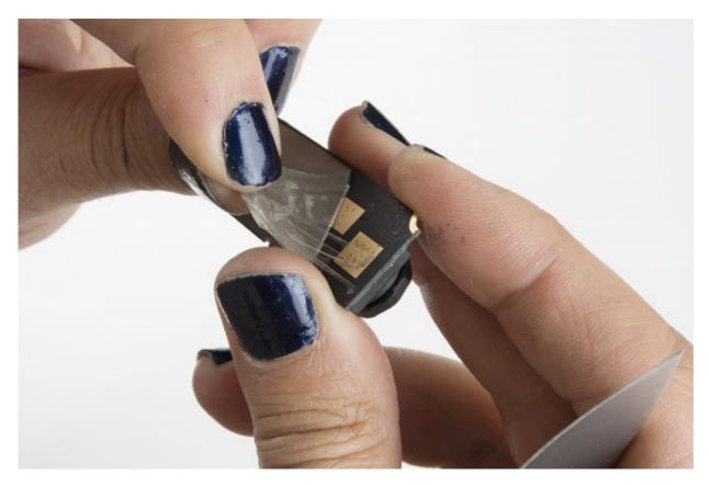
The back of the bottom PCB has a few bare copper pads visible through a conductive metal fabric. It would appear that the adhesive holding it on is either conductive or not designed not to be, so the pads and fabric probably allow for heatsinking to the case.
