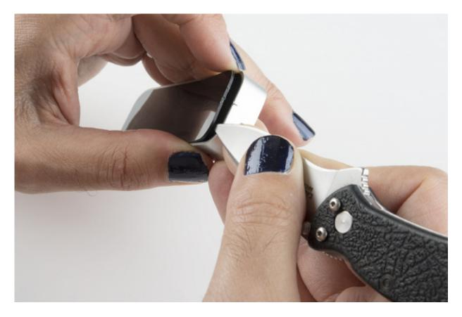
At first, I couldn't get enough of my knife-cum-spudger into the crack between the plastic and the case to make any real headway. I took a fine-tooth saw and cut a tiny notch in the case, and that was just enough to sneak the knife in and release some tension. After that, it was smooth sailing, except when I cracked the plastic a teeny, tiny bit.
