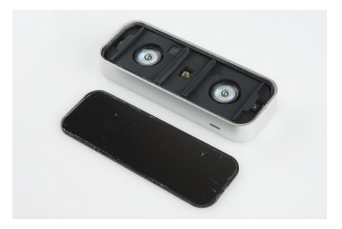
Finally, something interesting! Beneath the plastic is another rubber sheet, with holes for the three LEDs, two sensor elements, and one IC that was apparently a bit too thick to fit otherwise.
