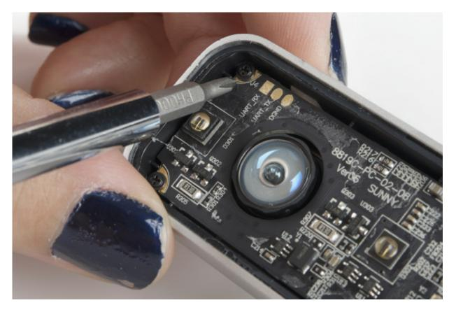
The third point of interest is the bare copper in the corners. I'm a little surprised to see that, as the screws on those points are black oxidized and they screw into a plastic holder, but it wouldn't surprise me if that's a throwback to an earlier version, or a "better-safe-than-sorry" sort of thing.
