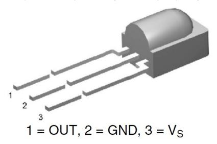
The IR receiver can be powered at anywhere from 2.5V to 5.5V, so it plays very nicely with a variety of development boards.
