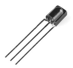
With three pins, it's about as simple as an IC can get. There are two pins for power -- ground in the middle, and & to a side -- and one, single data output pin.
