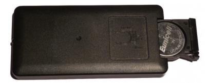
Insert the battery so that the positive (+) side is facing the bottom of the remote. Then slide the battery drawer back in.
