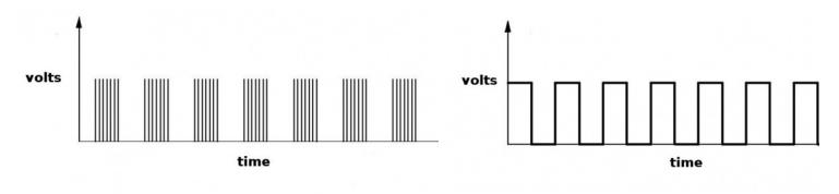
So all we have to do to read the output of this device is count high and low pulses, and measure their durations. For more information on the TSOP38238, check out its <u>datasheet</u>.
