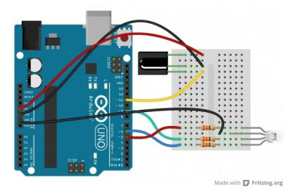
The output of the IR receiver connects to D11, but it could be connected to any digital input pin. If you swap pins, make sure you reflect those changes in code!
