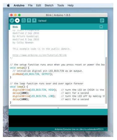
After a second, you should see some LEDs flashing on your Arduino, followed by the message Done Uploading" in the status bar of the Blink sketch.
