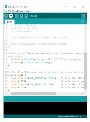
After a second, you should see some LEDs flashing on your Arduino, followed by the message Done Uploading" in the status bar of the Blink sketch.
