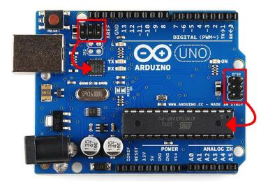
Here we have the Arduino Uno R3. It has two ICSP headers: one for the ATmega16U2 and one for the ATmega328. To reflash the bootloader on this board, you would use just the ICSP header for the ATmega328.
