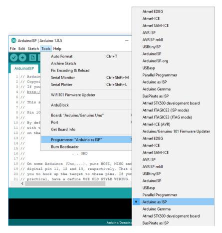
Heads up! You may encounter more than one selection for "Arduino as ISP" in the list of programmers. Either one will work. However, "ArduinoISP" will not work if it is selected.
