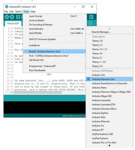
Select the programmer that you are using under**Tools > Programmer**. In this case, our programmer is an Arduino as ISP so select**Arduino as ISP**. You will also need to select the COM port that the Arduino as ISP is connected to if you have not selected the COM port already.
