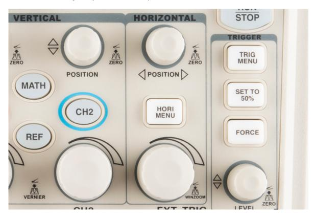
The **seconds per division** (s/div) knob rotates to increase or decrease the horizontal scale. If you rotate the s/div knob clockwise, the number of seconds each division represents will decrease – you'll be "zooming in" on the time scale. Rotate counter-clockwise to increase the time scale, and show a longer amount of time on the screen.
