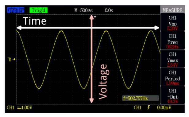
An example of an oscilloscope display. A signal (the yellow sine wave in this case) is graphed on a horizontal time axis and a vertical voltage axis.
