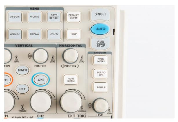
A series of buttons and screen menus make up the rest of the trigger system. Their main purpose is to select the trigger source and mode. There are a variety of **trigger types**, which manipulate how the
