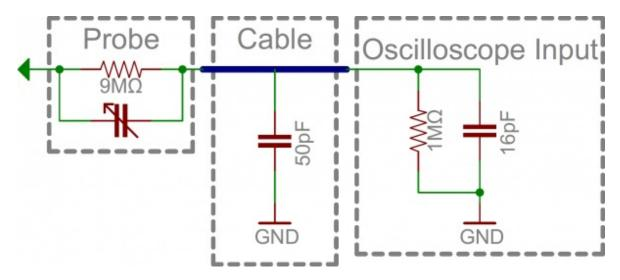
Most probes have a  $9M\Omega$  <u>resistor</u> for attenuating, which, when combined with a standard  $1M\Omega$  input impedance on a scope, creates a 1/10 voltage divider. These probes are commonly called **10X attenuated probes**. Many probes include a switch to select between 10X and 1X (no attenuation).
