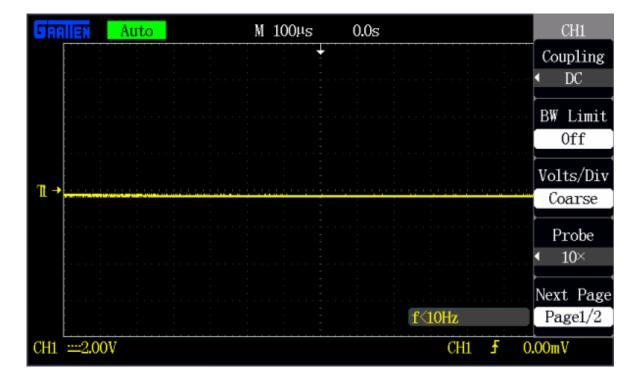
The screen should also show previously set values for time and volts per div. Ignoring those scales for now, make these adjustments to put your scope into a **standard setup**:
