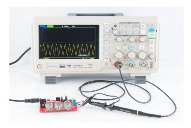
Once your signal is on the screen, you may want to begin by adjusting the horizontal and vertical scales into at least the "ballpark" of your signal. If you're probing a 5V 1kHz square wave, you'll probably want the volts/div somewhere around 0.5-1V, and set the seconds/div to around 100µs (14 divisions would show about one and a half periods).
