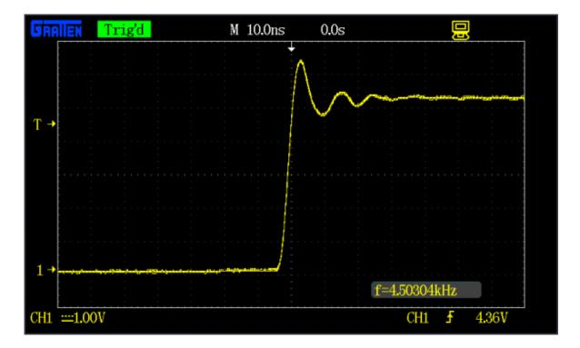
Using both the position and volts/div knobs in conjunction, you can zoom in on just a tiny part of the waveform that you care about the most. If you had a 5V square wave, but only cared about how much it was ringing on the edges, you could zoom in on the rising edge using both knobs.
