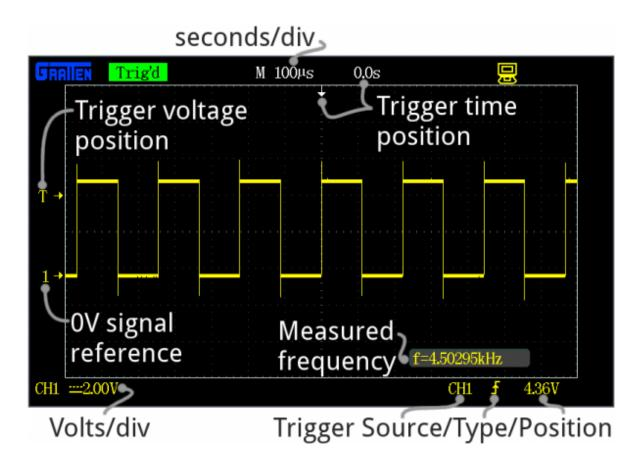
Every oscilloscope display should be criss-crossed with horizontal and vertical lines called**divisions**. The scale of those divisions are modified with the horizontal and vertical systems. The vertical system is measured in "volts per division" and the horizontal is "seconds per division". Generally, scopes will feature around 8-10 vertical (voltage) divisions, and 10-14 horizontal (seconds) divisions.
