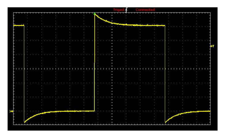
Adjust the trimming cap on the probe handle until you have a**straight-edged** square wave. Compensation is only necessary if your probe is attenuated (e.g. 10X), in which case it's critical (especially if you don't know who used your scope last!).
