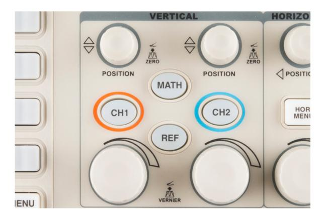
The more critical **volts per division** knob allows you to set the vertical scale on the screen. Rotating the knob clockwise will decrease the scale, and counter-clockwise will increase. A smaller scale – fewer volts per division on the screen – means you're more "zoomed in" to the waveform.
