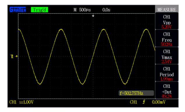
Using the scope's measure tools to find  $V_{PP}$ ,  $V_{Max}$ , frequency, period, and duty cycle.
