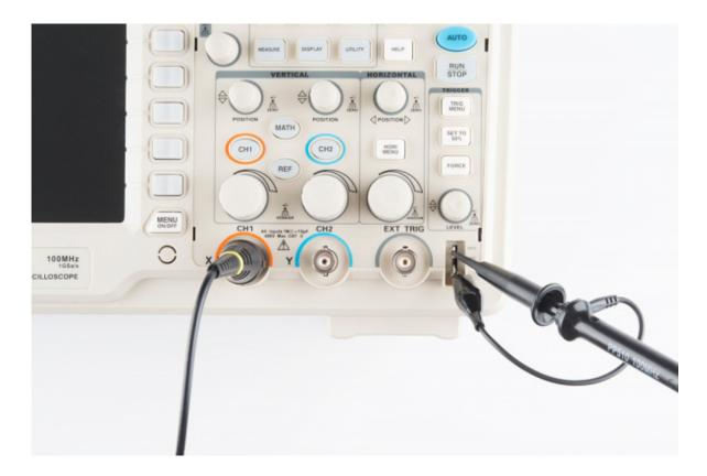
As soon as you connect both parts of the probe, you should see a signal begin to dance around your screen. Try fiddling with the **horizontal and vertical system knobs** to maneuver the waveform around the screen. Rotating the scale knobs clockwise will "zoom into" your waveform, and counter-clockwise zooms out. You can also use the position knob to further locate your waveform.
