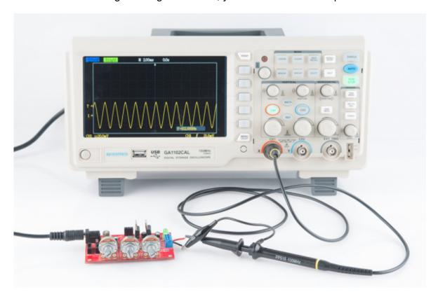
O-scopes are an important tool in any electrical engineer's lab. They allow you to see electric signals as they vary over time, which can be critical in diagnosing why your 555 timer circuit isn't blinking correctly, or why your noise maker isn't reaching maximum annoyance levels.
