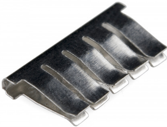
A single strip of conductive metal removed from the above breadboard.
