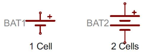
More pairs of lines usually indicates more series cells in the battery. Also, the longer line is usually used to represent the positive terminal, while the shorter line connects to the negative terminal.
