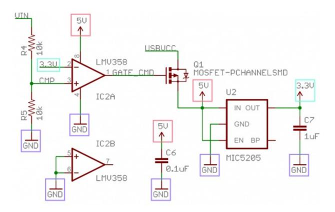
Like-named voltage nodes -- like GND, 5V, and 3.3V -- are all connected to their counterparts, even if there aren't wires between them.
