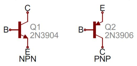
The collector (C) and emitter (E) pins are both in-line with each other, but the emitter should always have an arrow on it. If the arrow is pointing inward, it's a PNP, and, if the arrow is pointing outward, it's an NPN. A mnemonic for remembering which is which is "NPN: **n**ot **p**ointing i**n**."
