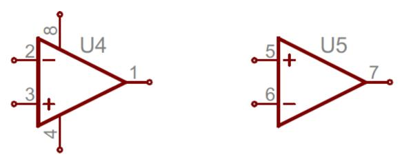
Often, there will be two op amps built into one IC package requiring only one pin for power and one for ground, which is why the one on the right only has three pins.
