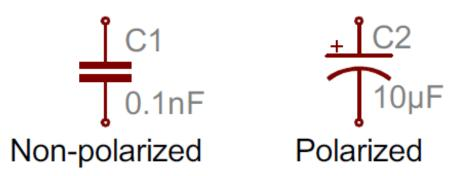
The symbol with one curved plate indicates that the capacitor is polarized. The curved plate usually Page 3 of 18
