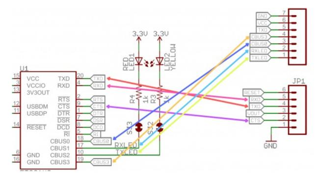
Each net with the same name is connected, as in this<u>schematic</u> for an <u>FT231X Breakout Board</u>. Names and labels help keep schematics from getting too chaotic (imagine if all those nets were actually connected with wires).
