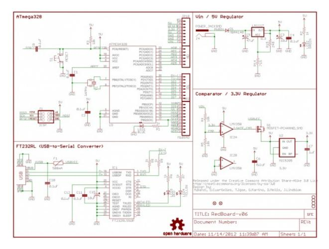
If the drawer of a schematic is really nice (like the engineer who designed this<u>schematic</u> for the <u>RedBoard</u>), they may separate sections of a schematic into logical, labeled blocks.
