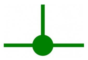
Nodes give us a way to say that "wires crossing this junction*are* connected". The absences of a node at a junction means two separate wires are just passing by, not forming any sort of connection. (When designing schematics, it's usually good practice to avoid these non-connected overlaps wherever possible, but sometimes it's unavoidable).
