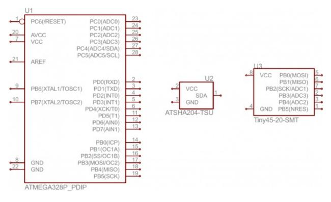
Schematic symbols for an ATmega328 microcontroller (commonly found on <u>Arduinos</u>), an ATSHA204 encryption IC, and an ATtiny45 MCU. As you can see, these components greatly vary in size and pin-counts.
