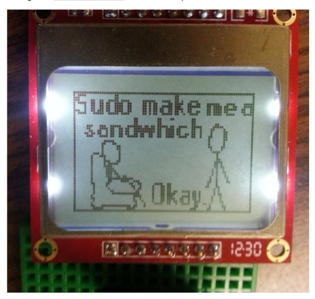
This is a demo of drawing bitmaps on the screen, which is one of the more rewarding tasks we can accomplish with the 'duino/LCD combo.
