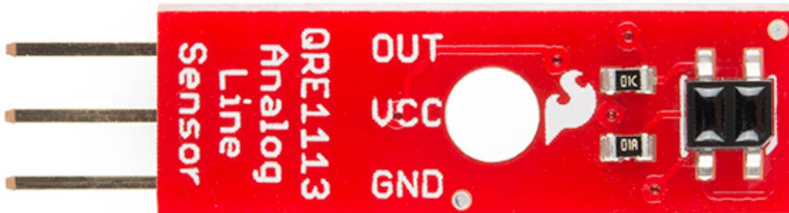
The Line Follower sensor is an add-on for your RedBot that gives your robot the ability to detect lines or nearby objects. The sensor works by detecting reflected light coming from its own infrared LED. By measuring the amount of reflected infrared light, it can detect transitions from light to dark (lines) or even objects directly in front of it.
