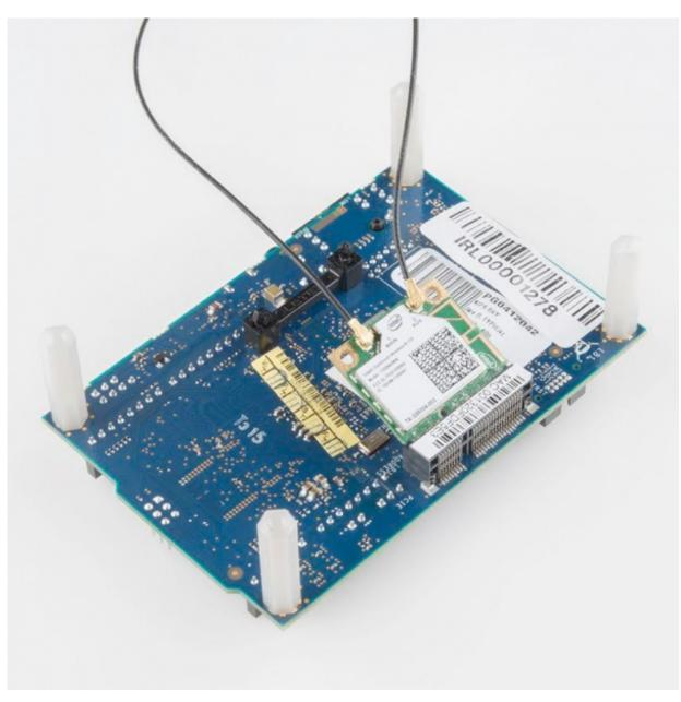
A half-size, mini PCIe WiFi card attached to the mating socket on the bottom side of the Galileo.
