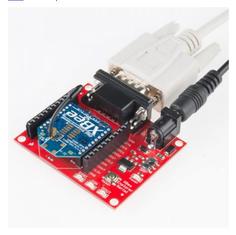
The Serial Explorer has a bigger footprint than its USB-based brethren, but still shares most of the same features. There are RX and TX LEDs, reset button, break-out pins, and a voltage regulator. One additional feature that the Serial Explorer has is an On/Off switch on board. This enables the user to turn on or off the power supply to the XBee module.
