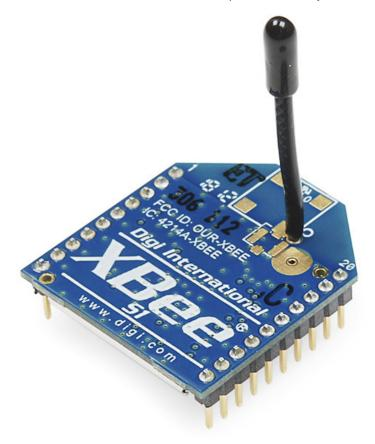
XBees are hugely popular wireless transceivers for a number of reasons. They'reflexible -- they send and receive data over a serial port, which means they're compatible with both computers and microcontrollers (like Arduino). And they're highly configurable -- you can have meshed networks with dozens of XBees, or just a pair swapping data. You can use them to remotely control your robot, or arrange them all over your house to monitor temperatures or lighting conditions in every room.
