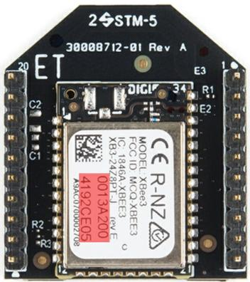
Each XBee has a unique MAC address, printed on a sticker in the highlighted area.
