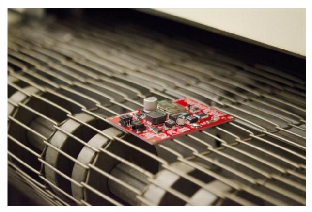
A populated board as it slowly enters the reflow oven Page 8 of 20 The reflow oven is kind of like a pizza oven. The board is raised in temperature to about 250°C (~480°F) at which point the paste turns to liquid metal. As the board exits the reflow oven, it quickly cools soldering all the components in place.
