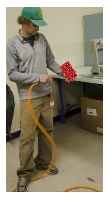
A fan or compressed air work well to remove any water that remains.
