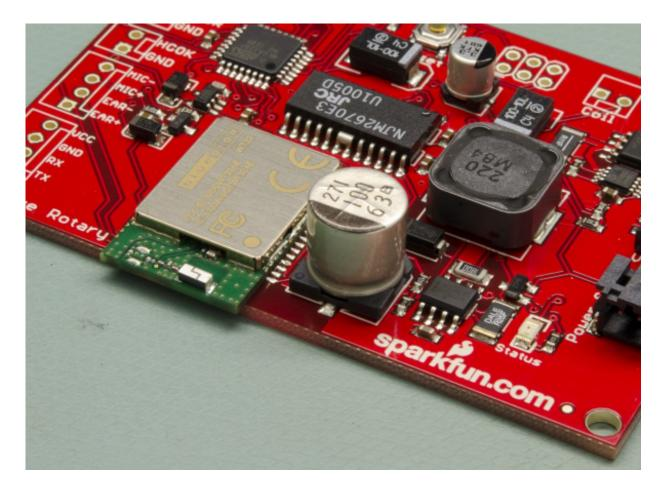
Cool to the touch, this board now has all the SMD components fully soldered to the PCB. The board is now ready for the next step!
