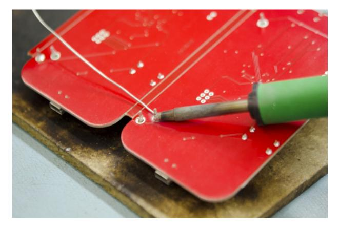
After reflow, a technician takes the board and manually solders any PTH (plated through-hole) components. In a larger production facility, the soldering of through-hole components may be done using a technique known as <u>wave soldering</u>, where the board is passed over a standing wave of molten solder, which adheres to component leads and any exposed metal on the board.
