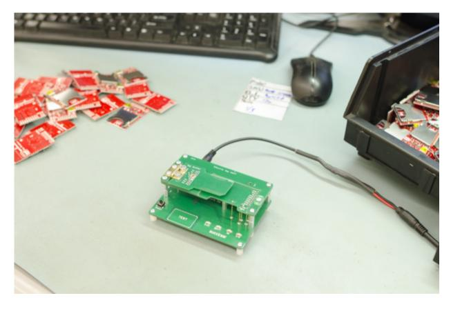
Once the board has been inspected it is tested to make sure it does what it is supposed to do.
