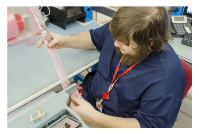
Once the batch of boards is clean and dry, they go to packaging where each board is individually heat sealed into ESD plastic.
