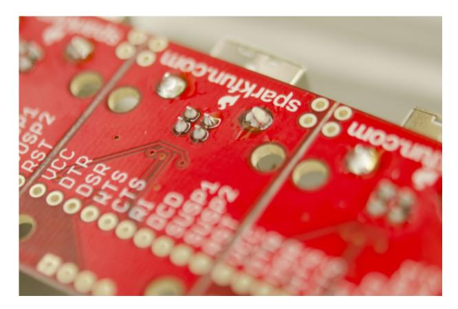
Various steps of the manufacturing process leave residue on the board. If you've ever pubne of <u>our kits</u> together, you know that soldering leaves a small amount of flux on the board. Over a period of months this flux residue becomes sticky, looks horrible, and can become slightly acidic leading to a weakening of solder joints. To prevent this (and to give our customers the best looking boards) we wash every board we produce.
