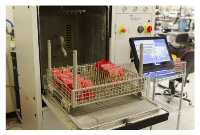
To get the boards clean again we load batches into what we call the 'dishwasher'. This high temperature, high pressure, all stainless steel dishwasher uses deionized water to remove any residue from the manufacturing process.
