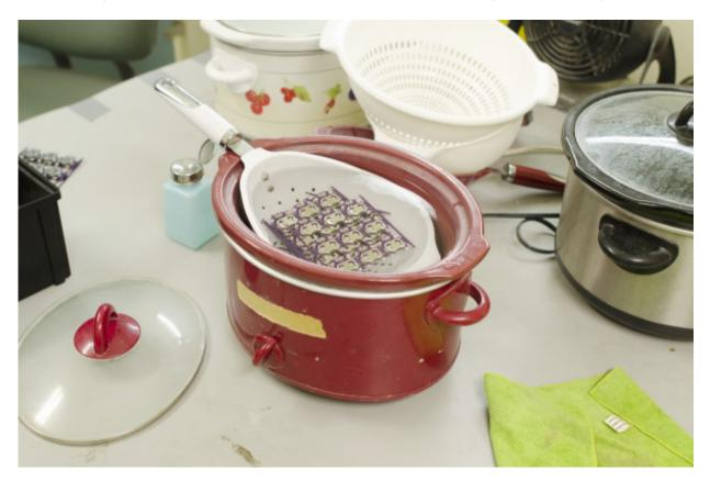
Don't have access to an expensive washer? A cheap crockpot with deionized water and a toothbrush work swimmingly! If you're cleaning just a few boards, a Q-tip with some isopropyl alcohol works very well.
