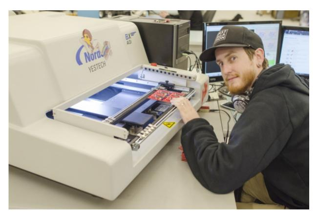
The next step is optical inspection. Optical inspection catches any problems with parts (wrong
