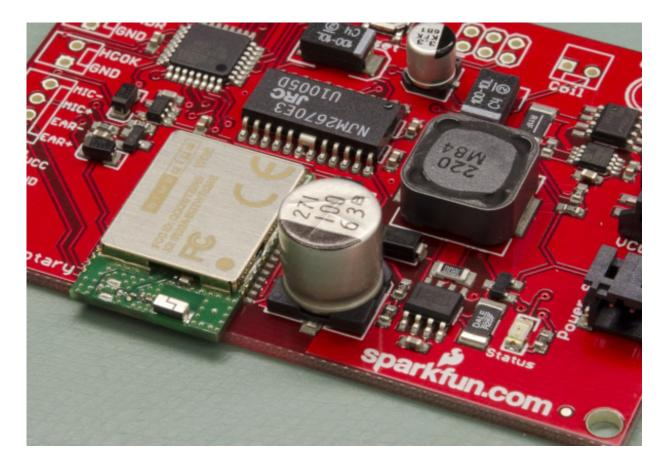
Here we have the control board for the infamous <u>Portable Rotary Phone</u> with components placed on the solder paste. The paste is tacky like butter sticking to a dish. The components stay in place while the board slowly moves through the reflow oven.
