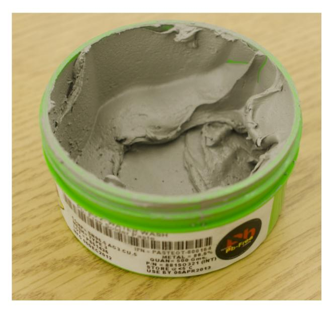
This is what solder paste looks like in the wild. It's a mixture of metal alloys: 96.5% tin (Sn), 3% silver (Ag), and 0.5% copper (Cu). Most paste has an expiration date and should be stored in a cool place. This has to do with the flux that is added to the metals thus creating the paste consistency. Flux changes the surface tension of the metal when it is in liquid form helping it to flow into the joints.
