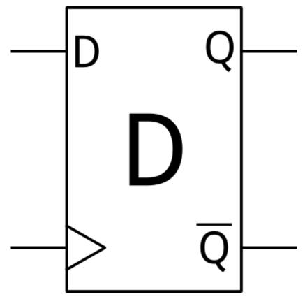
The simplest type of flip-flop is the D-type. D flip-flops are simple -- upon a clock edge (normally rising, although they can be found with a built-in inverter to clock in on the falling edge instead), the input is latched to the output.
