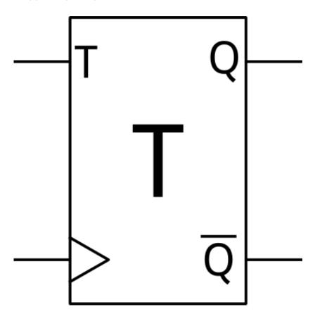
Only slightly more complex is the T-type. The 'T' stands for "toggle." When a clock edge occurs, if the input T is a 1, the output changes state. If the input is a 0, the output remains the same. As with the D-type, the complement of the output is usually provided.
