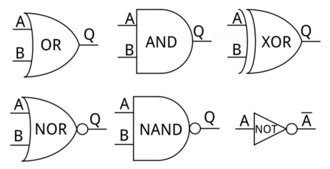
Combinational circuits are built of five basic logic gates:
