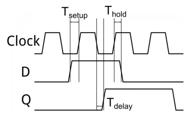
Note that in the above image, transitions are drawn as being slightly angled. This serves two purposes: it reminds us that clock and data edges are *never* truly right angles and will always have some non-zero rise or fall time, and it makes it easier to see where the vertical lines marking the various times intersect with the signals.
