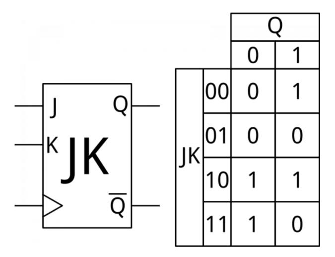
Finally, we have the JK-type. The JK-type is the only one of the three which truly requires a truth table to explain; it has two inputs (J and K), and the output can be left the same, set, cleared, or toggled, depending on the combination of input signals present. Of course, as with all flip-flops, the input at the moment of the clock is the only thing that matters.
