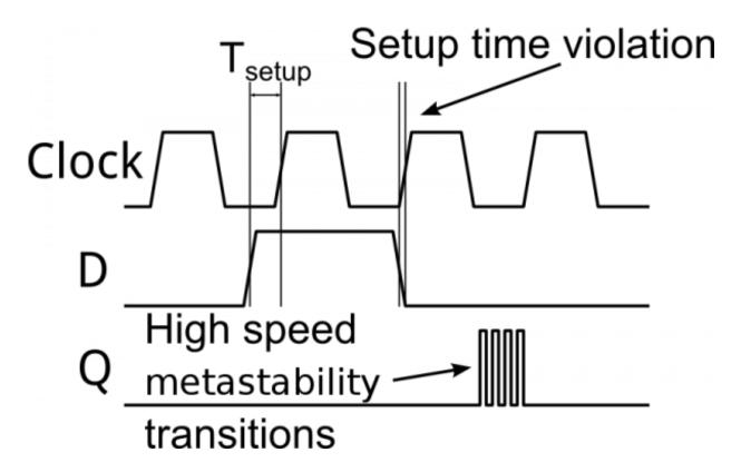
Metastability problems can range from spurious operation up to damage of the chip, since they can increase current consumption. While metastability usually resolves on its own, by the time it does so, the system may be in a totally unknown state and need to be completely reset to restore proper operation.
