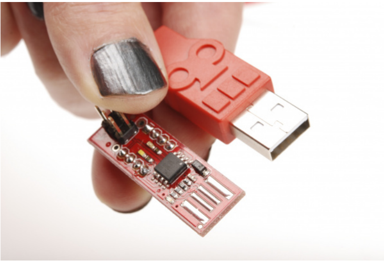
Two types of Male USB-A connectors, on a SparkFun Cerberus cable and an AVR Stick development board.
