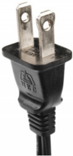
A polarized North American wall plug. By having two different widths for the plug blades, the plug will only go into the outlet one way.
